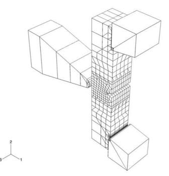
FIGURE 2. The finite element mesh of the Charpy specimen, the anvils and the striker.
