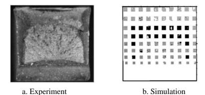
FIGURE 5. Experimental (a) and simulated (b) Charpy fracture surfaces. In (b) the black colour denotes brittle fracture and grey, the ductile fracture.
