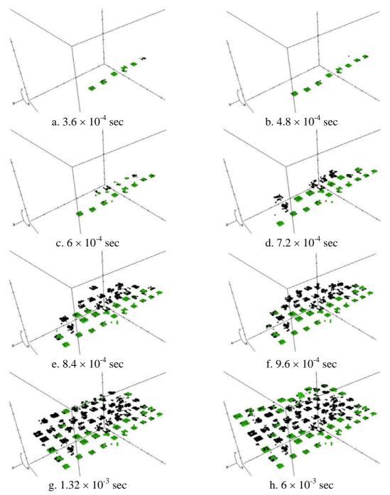
FIGURE 4. Fracture propagation on the CA scale at –30°C. Only dead brittle (black) and dead ductile (green) cells are shown.
