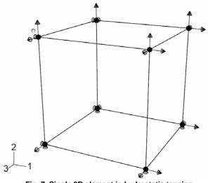
Fig. 7. Single 3D element in hydrostatic tension
