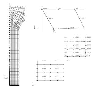
Fig. 10. Finite element model of round bar
