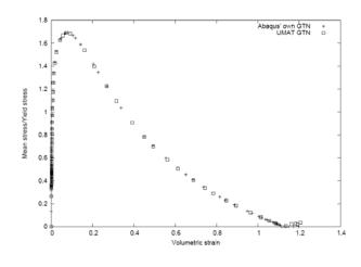
Fig. 13.Plot of  $\sigma_{_{m}}/\sigma_{_{PL}}$  versus volumetric strain  $arepsilon_{_{ii}}$
