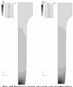
Fig. 15.Contour plots of void volume fraction
