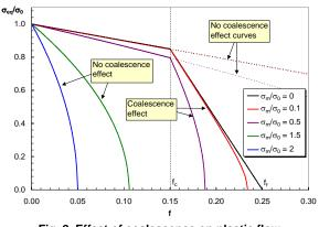
Fig. 2. Effect of coalescence on plastic flow for different values of hydrostatic stress
