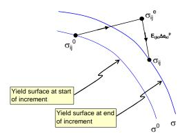
Fig. 3 construction of new stress tensor during yielding
